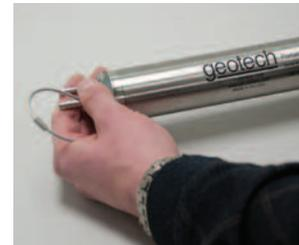
Replace the outer housing (21150041). Be sure the outer housing is sealed against the upper cap.
