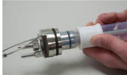
Slide a Teflon® compression ring (#11150042) over the bladder and push down over bladder and upper end of the center tube.
