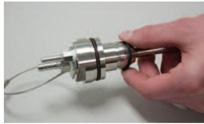
Slide bladder onto the center tube assembly and over the O-ring (#11150319) on the upper end of the center tube assembly. Be careful not to roll the O-ring when sliding the bladder over this end.
