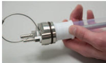
With the upper end of the bladder secured by the Teflon® compression ring, slide the second compression ring over the bladder about mid-way down the assembly.
