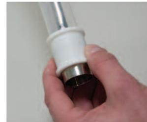
Slide the bladder back down over the O-ring being careful not to roll the O-ring.
